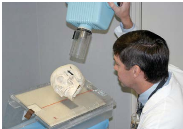
FIGURE 27-11 Practicing beam angulation on a dry skull is an excellent way to learn transcranial radiography.
